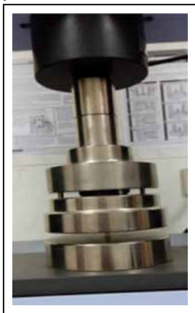
Fig. (2): Universal testing machine used for compressive strength testing
