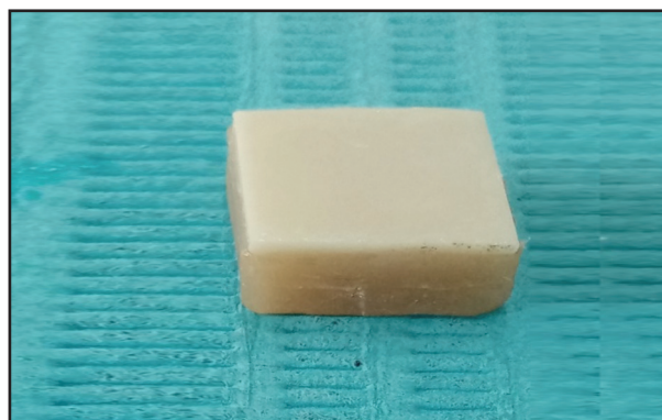
Figure (1): Ceramic veneer cemented to composite resin substrate
