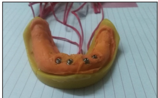
Figure (4): Strain gauge installed
