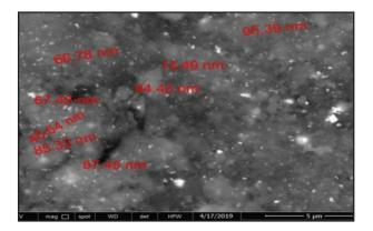
Figure (1): Scanning electron micrograph for the prepared MMT-AgNPs powder
