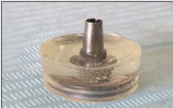
Figure (1) Implant and implant abutment embedded in epoxy resin
