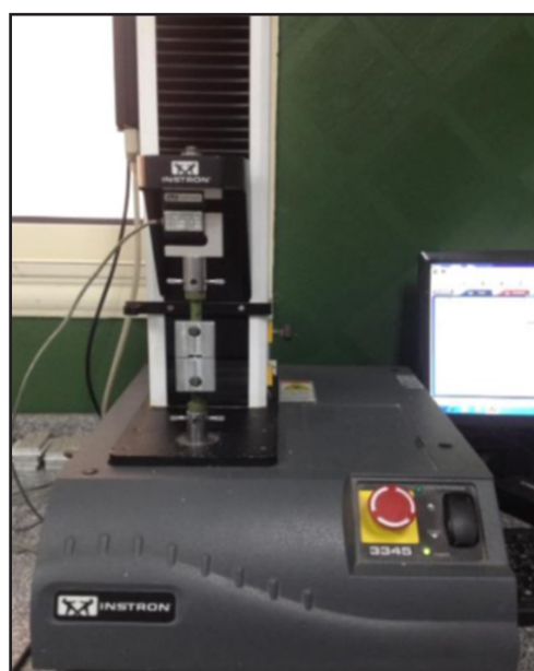
Figure (1) Jig mounted and parallel aligned on the Universal testing machine.
