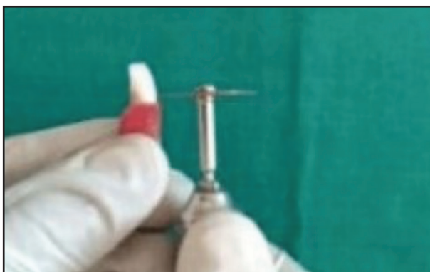
Figure (1) Sample preparation by separation of the root at the CEJ using a diamond disc.
