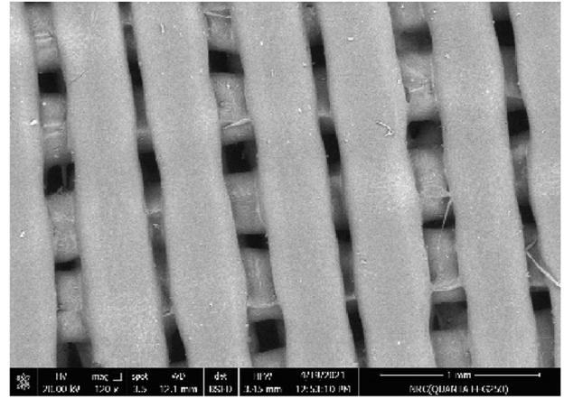
Fig. 6. SEM image of unmodified scaffold surface after cell attachment.
