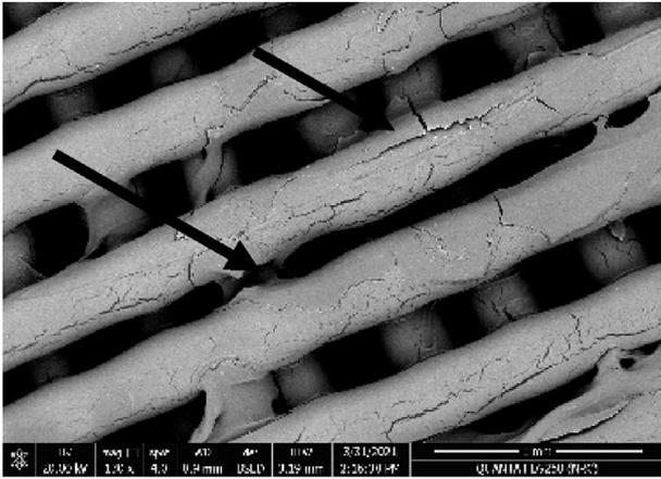
Fig. 3. SEM image showing the scaffold surface of group B.
