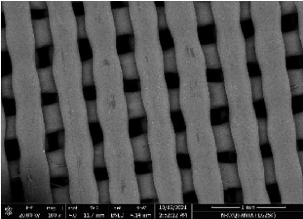
Fig. 4. SEM image showing scaffold surface of group C.
