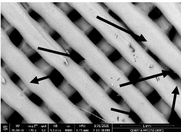
Fig. 5. SEM image of modified scaffold surface after cell attachment.
